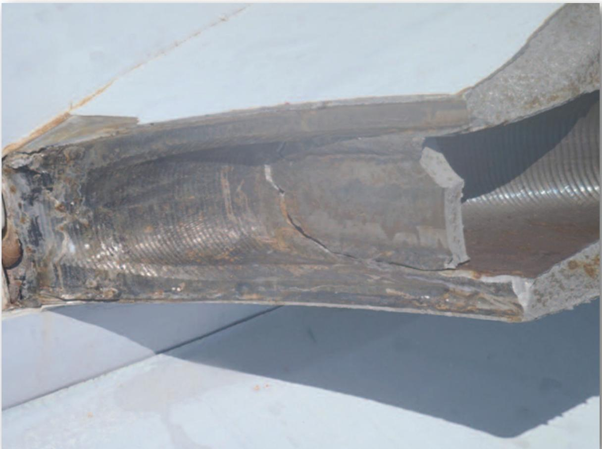
Appendix 7.4 Photos of 'Rambler 100' Inverted showing Failed Keel Stub.
