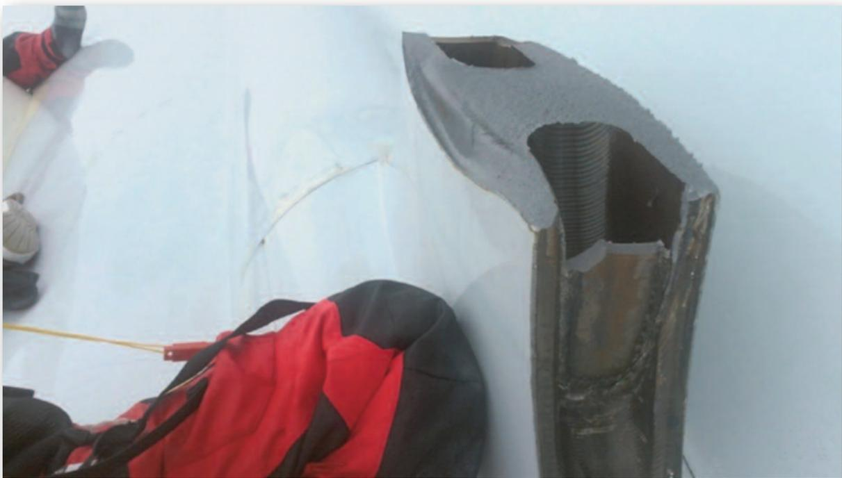
Appendix 7.4 Photos of 'Rambler 100' Inverted showing Failed Keel Stub.
