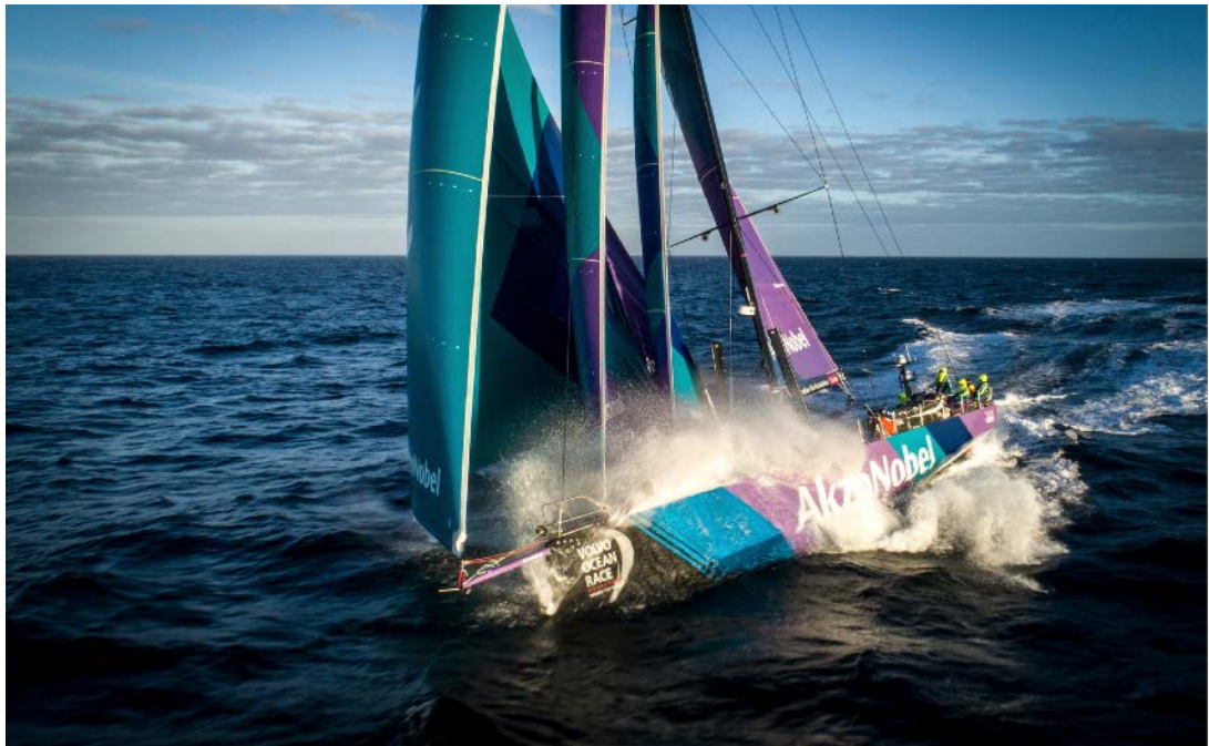
Figure 14- Akzonobel with the radar antenna visible on the mast just above the top of the daggerboards - the steaming light can be seen on the mast just above the spreaders
