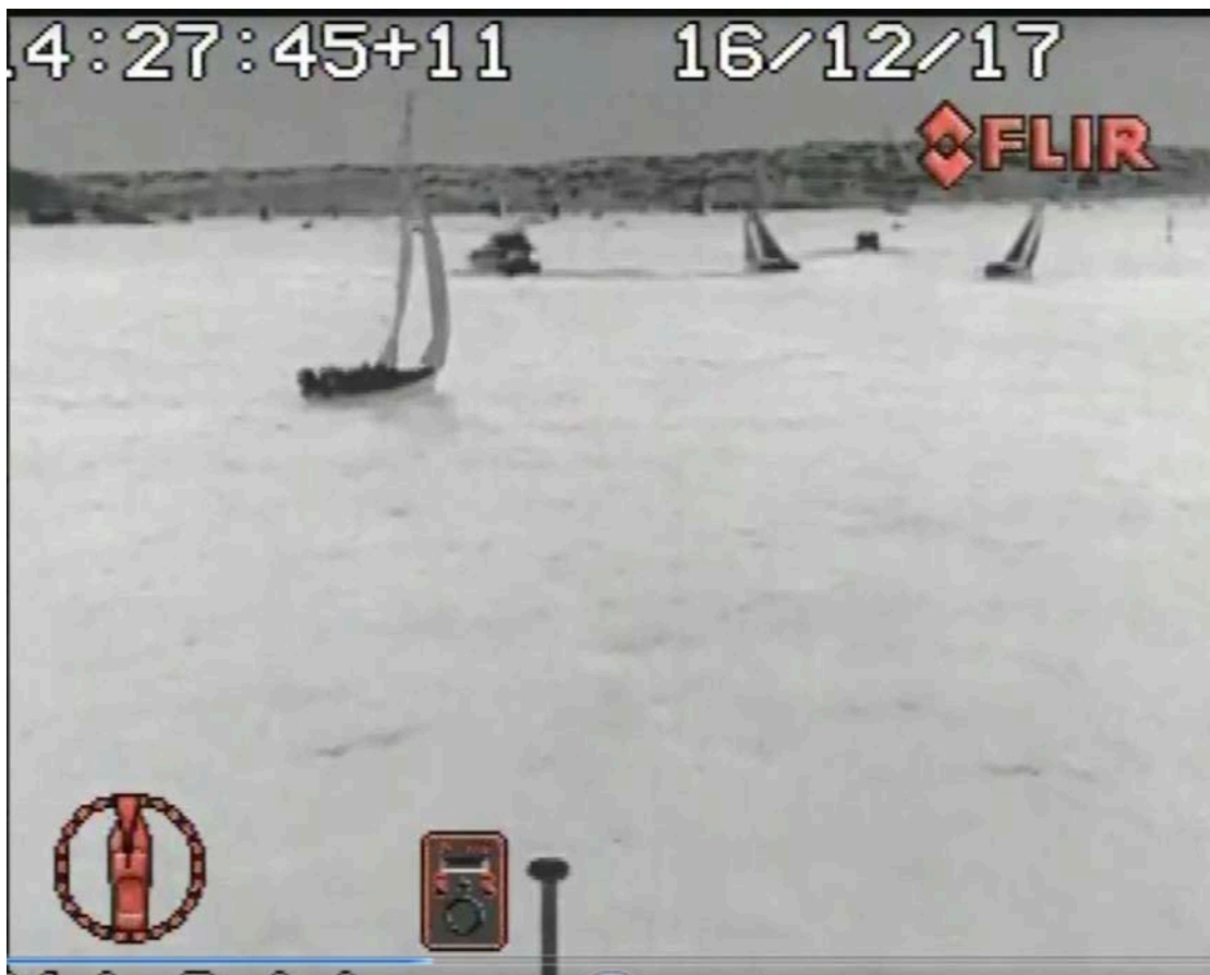
Figure 19 - Daylight FLIR screen from a Manly Ferry on Sydney Harbour - Headland (Right Hand Edge) at top left of screen is 1.2nm, land beyond is at a distance of 2-3nm
