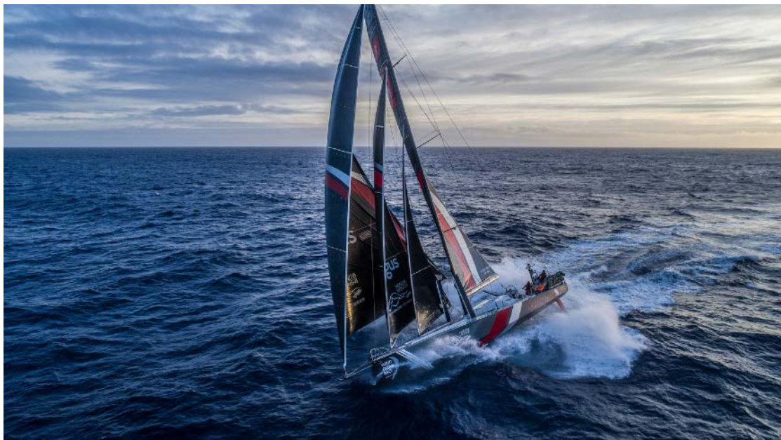
Figure 7 - Sun Hung Kai/Scallywag sailing with a triple headsail rig - MH0, J2 and J3 - the MH0 is sheeted through a outrigger Credit: Konrad Frost / Volvo Ocean Race
