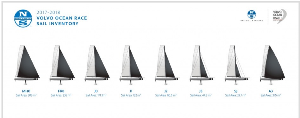
Figure 6 - The VO 65 headsail sail plan
