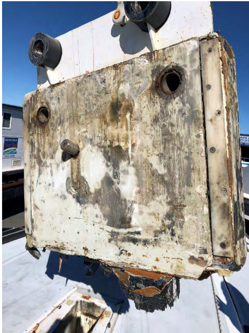
Picture 2 - Remains of keel as extracted from hull.
