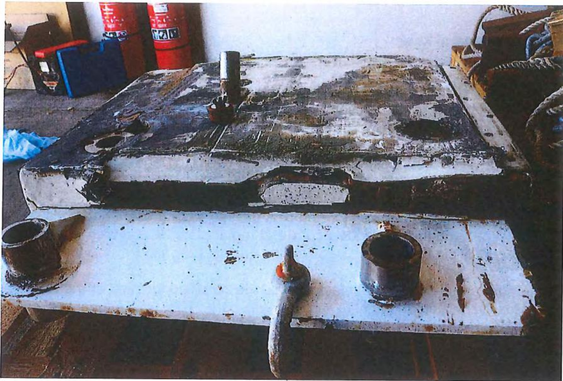
Image 10, shows externally visible damage to the port side of the keel. The wooden core has dropped, and the anti-gravity pin has been pulled through to the port side. Deconstruction would later confirm that extensive de-lamination (of the wooden core, steel/epoxy interface, through keel fittings and external keel skin) had occurred causing the port side skin to slip.
