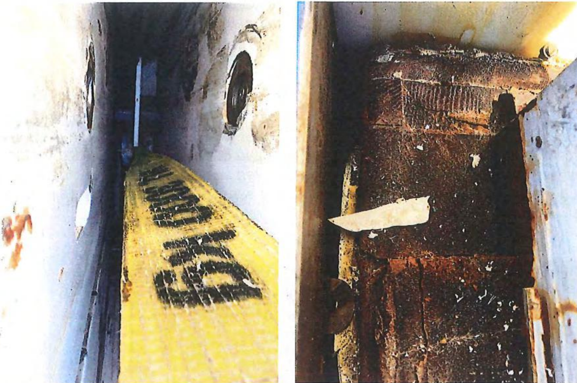
Image 16-17, Keel inside the keel box viewed from the top. note: damage is evident on the port side of the keel.
