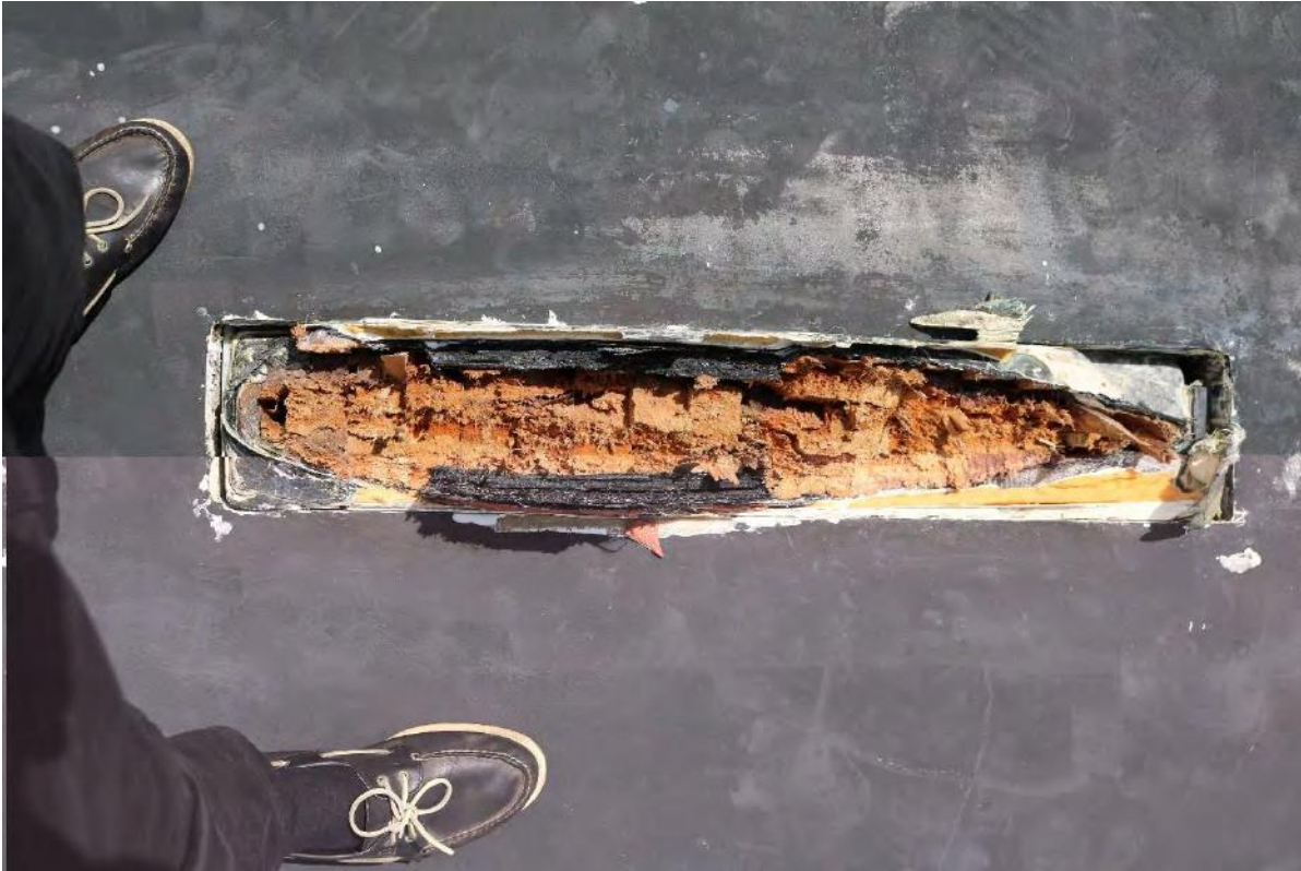
Picture 1 - Remainder of keel flush with underside of salvaged hull.
