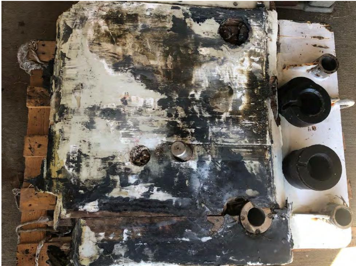
Picture 3 - Port skin moved down relative to remainder of keel.
