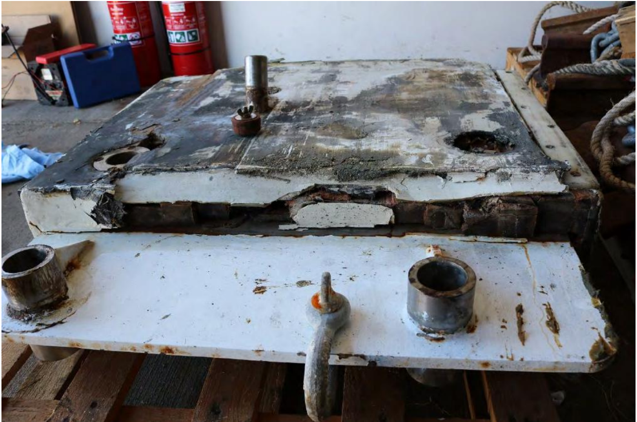
Picture 4 – Core failed in shear, outside skin moved relative to remainder of keel.
