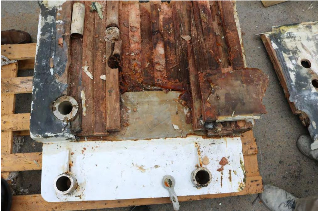
Picture 5 – Outside skin of keel removed, evidence of water ingress and degradation of core.
